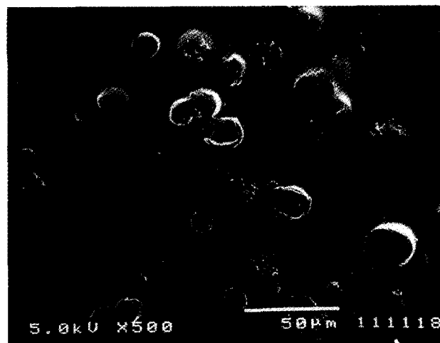
Figure 5 SEM images of (a) pure LDPE, (b) LDPE + 7.7% starch and (c) LDPE + 20%MB. Left-hand side, unaged samples; right-hand side, samples thermo-oxidized for 42 days
